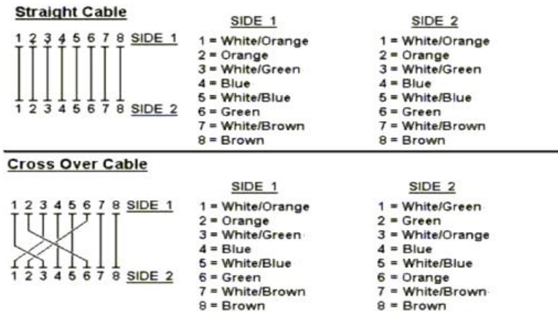
Figure A-1: Straight-Through and Crossover Cable
